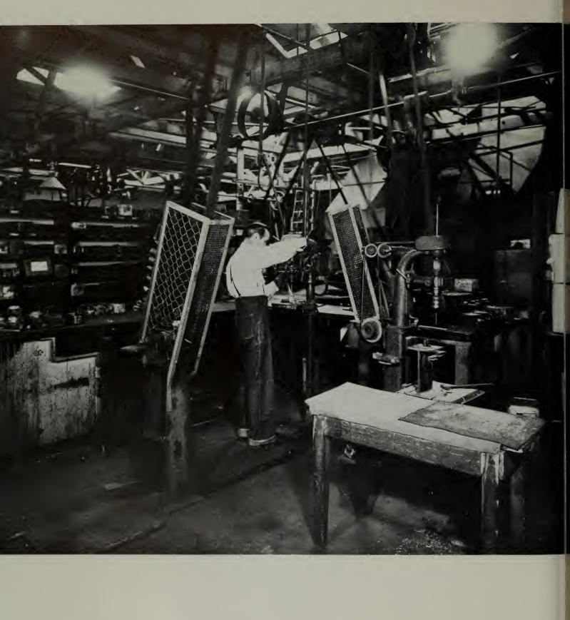
The operator cleans out the oil holes by use of a drill press as shown in this picture.
